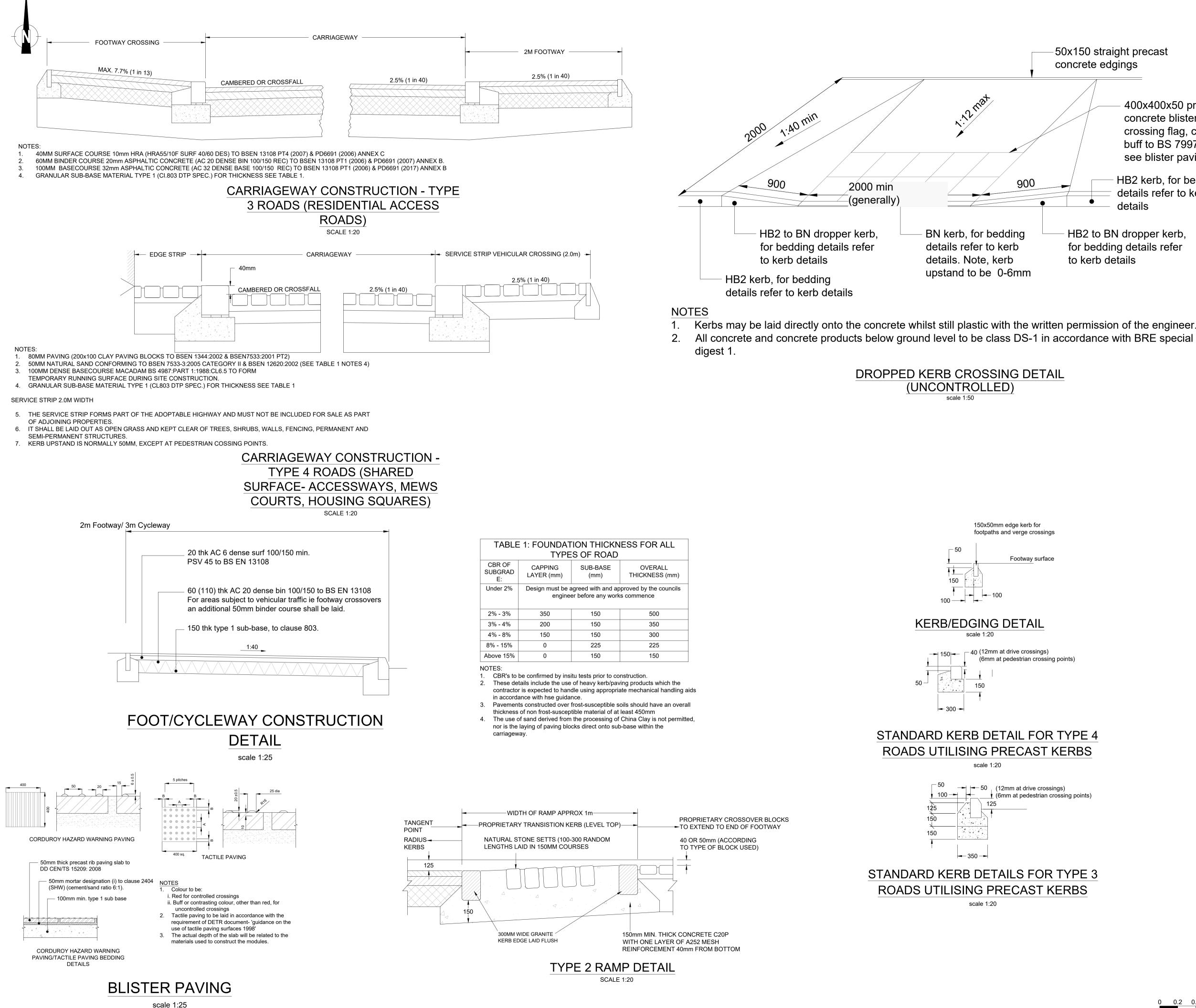
All concrete and concrete products below ground level to be class DS-1 in accordance with BRE special
